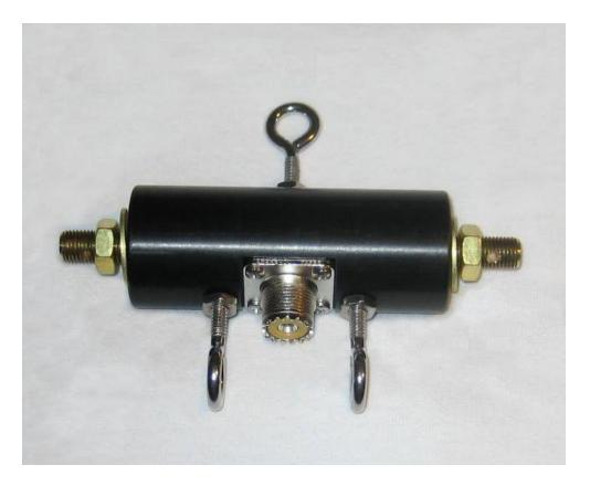
The body is machined from a billet of DuPont Delrin using custom tooling. It includes two 3/8-24 threaded female connectors to accept threaded rods for wire antennas and stick antennas. An Amphenol 83-1R SO-239 is used for legal-limit operation. Pricing is located below, after a brief review.
